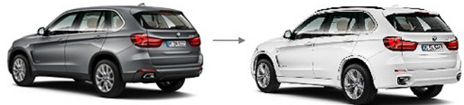
Comparison of X5 without and with the M Aerodynamics basic package retrofit kit
